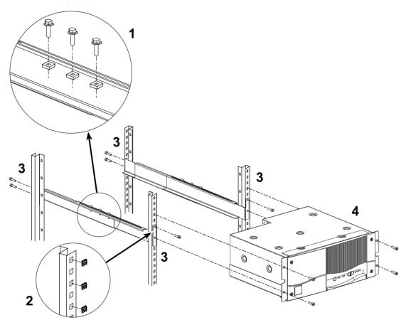
The rails and the necessary mounting hardware are supplied with the **UPS** in the package.
